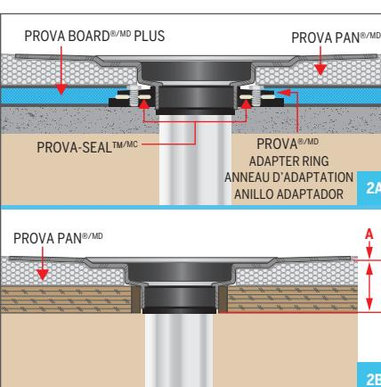
The following instructions will guide you through the installation of PROVA DRAIN<sup>®</sup> PLUS. For installations of the drain without the included adapter ring, which is optional and used for connecting to existing three-piece drains, begin at step 2B. For installations with the adapter ring, begin at step 1.
