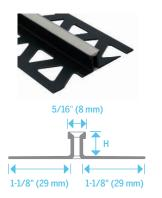
Co-extruded from rigid and flexible PVC, the Expansion Joint profile is perfect for use in tiled floor applications where flexibility is required to account for substrate movement. Ideal for use in lightduty commercial applications to protect tile from cracking. Resistant to weather, UV rays, and most household cleaning products.
